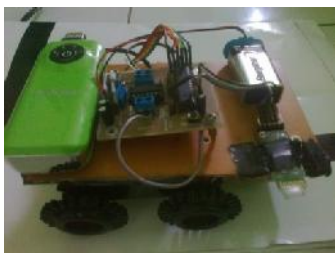
Gambar 14 Hasil akhir robot line follower
